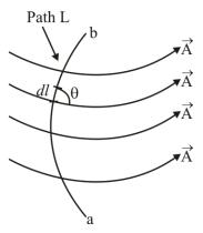
If path of integration is closed curve then it becomes a closed contour integral, which is called the circulation of **A** around **L**. and defined as
